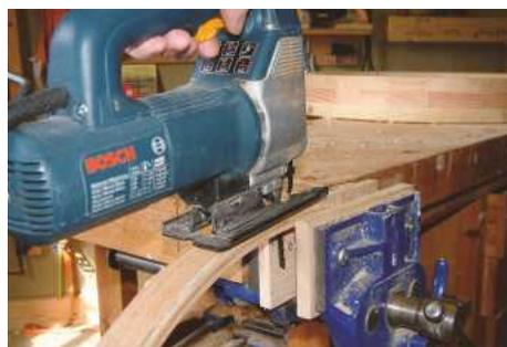
▲ Pic.13 Cut the beading to width with a jigsaw, cleaning up the surfaces with a block plane
